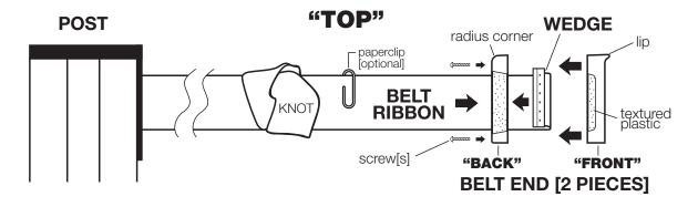
**BEFORE YOU START:** Examine your new plastic Belt End carefully. It will arrive disassembled in two pieces. **Belt End "BACK":** Has textured plastic that wraps around the back and a radius corner which should be oriented to "TOP".
