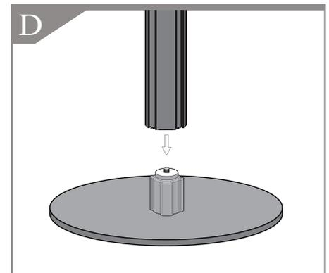
5. On bottom of the base: Use supplied Allen Wrench (5/16 drive) to tighten the center Hex Bolt. **Tighten minimum of 5 turns** with at least 20 ft–lbs of torque. See Figure E.
