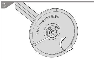
**ATTENTION:** Over time, extensive handling of the stanchion may cause the rubber insert that holds the base to the post to loosen slightly. Should this happen, please use an Allen Wrench (5/16" Drive) to tighten the bottom hex bolt.
